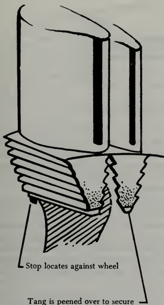
FIGURE 1-55. Turbine bucket, featuring tang method of blade retention.
